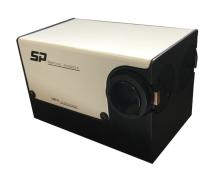
Single-piece base construction, direct grating drive, and anti-backlash gearing ensure this unit is rugged and stable enough for demanding applications. Loaded with SP Optics and able to hold two high-quality gratings, the CM110 is ideal for spectrometry in the UV to IR spectra. Each instrument is calibrated and certified before delivery and comes with easy-to-use software.
