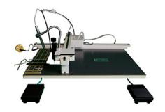
eC-placer is a camera-assisted manual pick and place device designed and priced for prototype and small series assembly.
