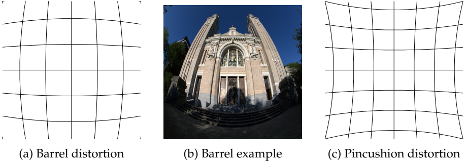
Figure 2.4: The projective geometry of a camera is disturbed by geometric aberrations of the lens, which should be cancelled.
