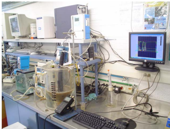
Figure 1 Automated pilot reactor utilized for 4CP degradation
