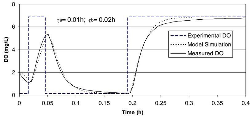
**Figure 5** Experiment for identifying DO sensor. The dashed straight line is the real oxygen to which the probe was exposed (by quickly changing it from one beaker to another with opposite DO conditions). The continuous line is the sensed signal. The dotted one is the model simulation
