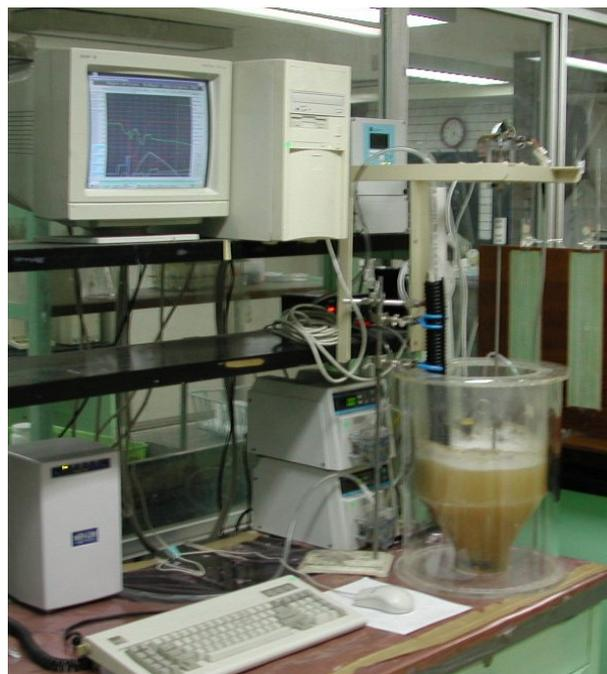
**Figure 1** Pilot reactor utilized for the toxic compounds degradation
