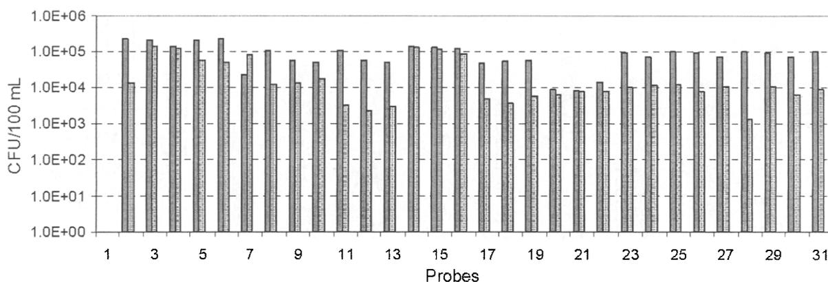
Fig. 1. Evolution of the faecal coliforms in the system with 10% urban wastewater in the feed (■ influent SBR, □ effluent SBR previous to filtration).
