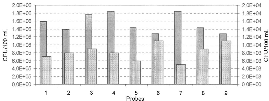
Fig. 3. Evolution of the faecal coliforms in the system with 100% urban wastewater in the feed (■ influent SBR, left axis; □ effluent SBR previous to the filtration, right axis).
