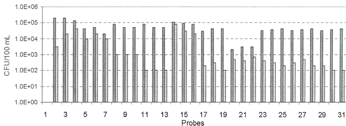
Fig. 2. Evolution of the *E. coli* in the system with 10% urban wastewater in the feed (■ influent SBR, □ effluent SBR previous to the filtration).
