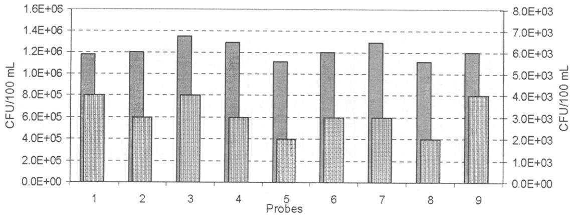
Fig. 4. Evolution of the *E. coli* in the system with 100% urban wastewater in the feed (■ influent SBR, left axis; □ effluent SBR previous to the filtration, right axis).
