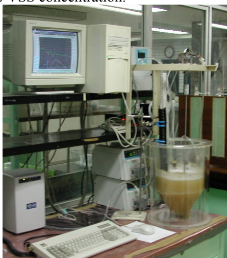
Figure 2 Pilot reactor utilized for the toxic compounds degradation
