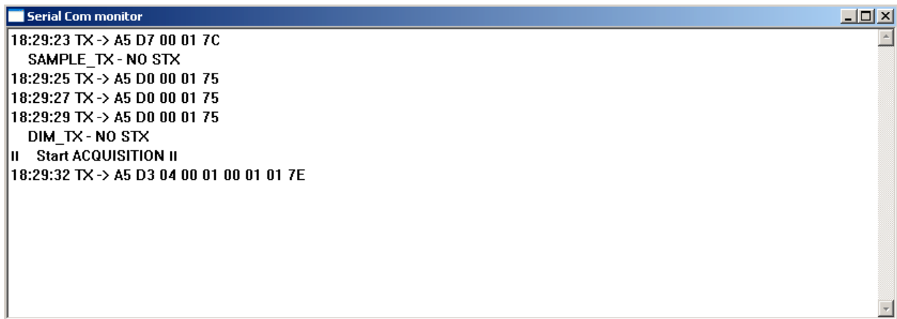
Figure 2.1 - view RS232 hexadecimal packets
