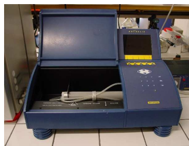
Figure 3.4.1. The Anthelie spectrophotometer (Secomam).
