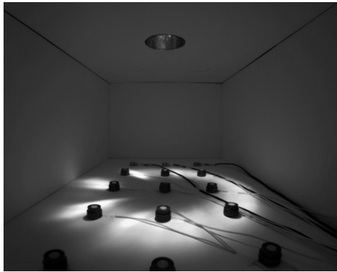
Figure 10: Illuminance sensors in a scale model.
