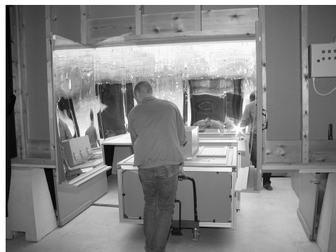
Figure 6 : The mirror box doors width fixes the maximal scale model dimensions.
