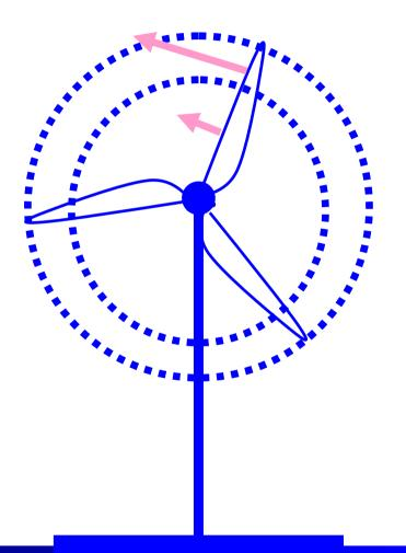
Due to high speed, wing tips are most efficient part of wing
