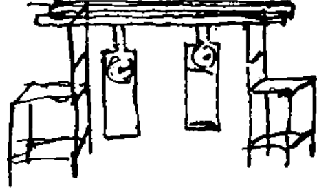
Fig. 5. The Huygens drawing describing his synchronization experiment
